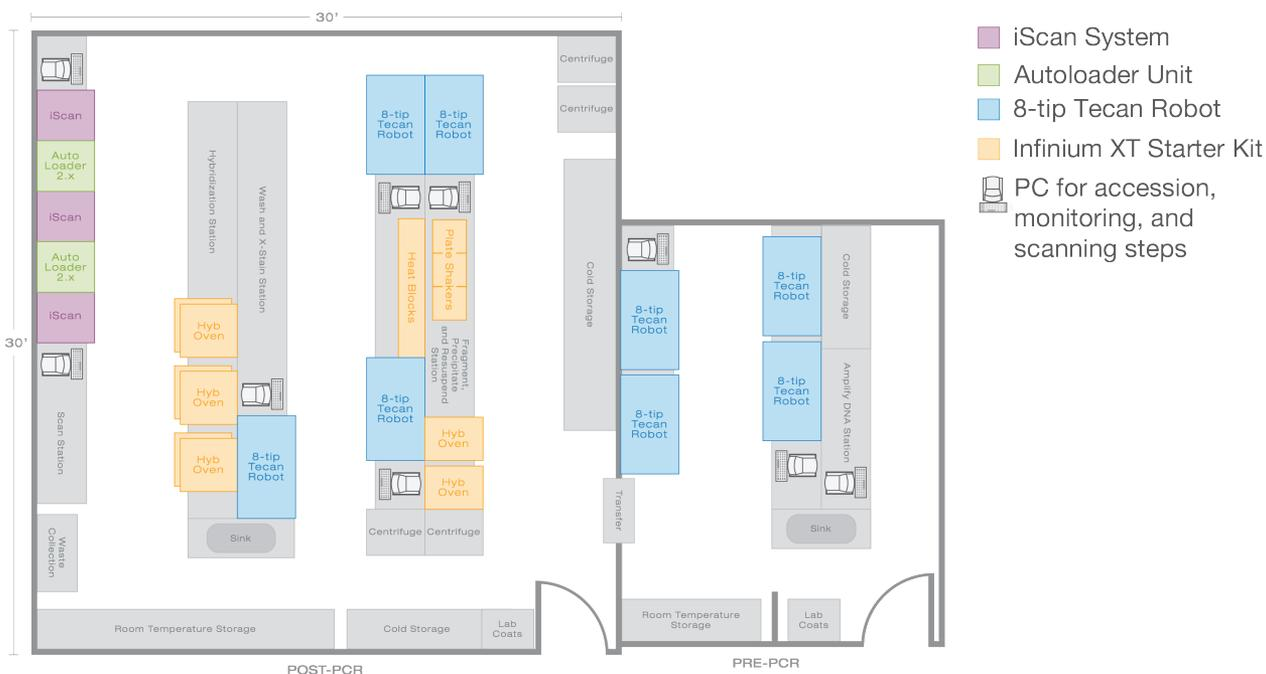
**Figure 4: Example Lab Layout for Infinium XT Production-Scale Genotyping**—An example lab layout is provided for processing 1,000,000+ samples per year and includes: three (8-tip) Tecan robots, three iScan Systems, two AutoLoader 2.x units, and ancillary lab equipment. This example layout requires approximately 1200 square feet. Layout is not to scale.
