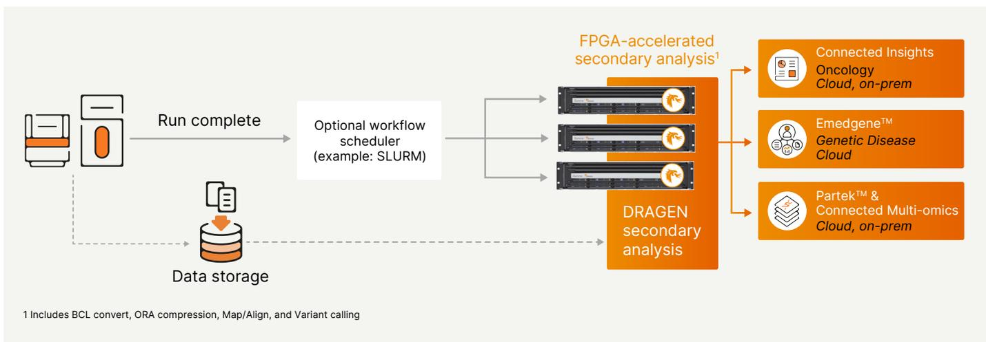
Figure 1: Example on-premises workflow, including instrument connection, optional workflow scheduler, analysis, and interpretation.
