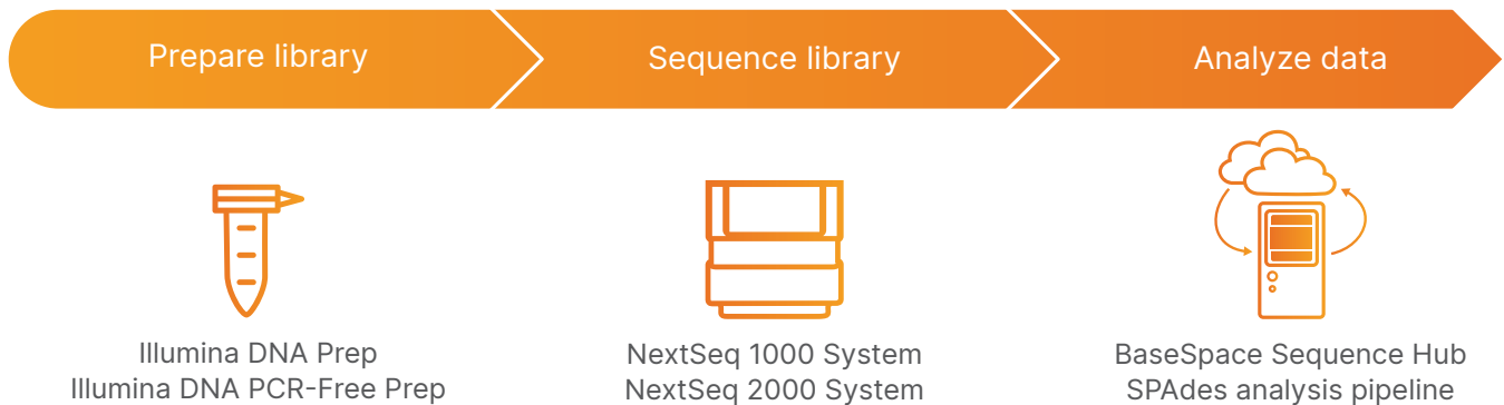
Figure 1: WGS workflow on NextSeq 1000 and NextSeq 2000 Systems—The user-friendly streamlined NGS workflow includes library prep, sequencing, and data analysis. Sequencing run time for the NextSeq 1000/2000 P1 Reagents (600 cycle) flow cell is ~34 hr and run time for the NextSeq 1000/2000 P2 Reagents (600 cycle) flow cell is ~44 hr.
